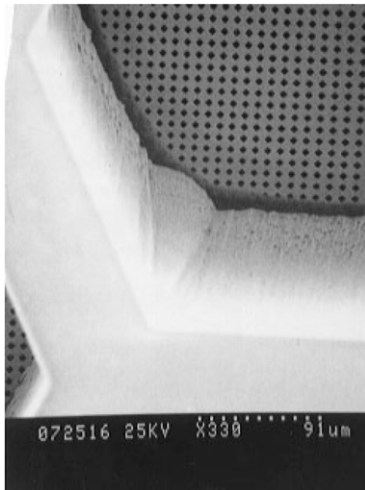
Figure 8. Microporous gas diffusion layer formed in the silicon membrane at the bottom of flow field channels by DRIE. The pore diameter is 4\ \mu\text{m} and the silicon membrane thickness is 80\ \mu\text{m} .
